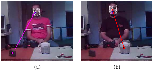
Fig. 10. Estimated gaze direction and object depth via GP regression (line) together with the center of the manually annotated object of interest (solid dot).
