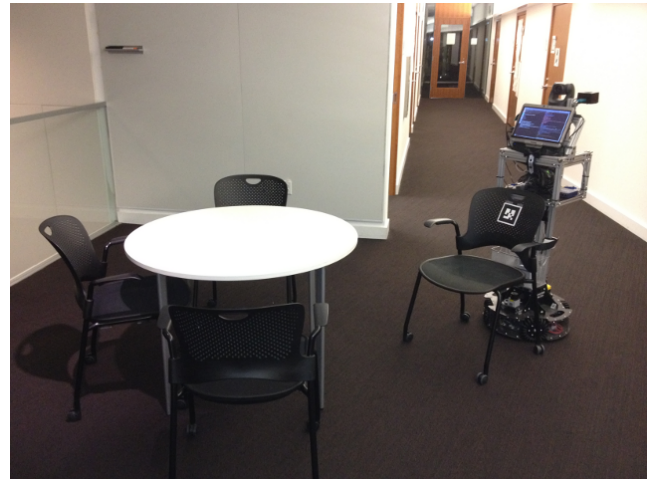
Figure 6: A snapshot from one of the real world experiments. The chairs and the robot almost perfectly match the models used in simulation. In order to make the perception of the chair easier, we placed AR tags on both sides of the back of the chair. The robot uses its global localization estimate to compute the global poses of the other objects in the environment and construct its world model.
